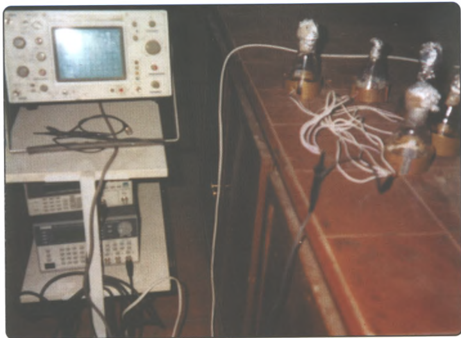
Fig. 1. MHz synthesized ARBitrary wave generator attached with flasks containing YES medium inoculated with A. flavus spores.
